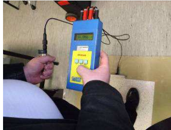
Deposited on a conductive surface ESD PVC PU sealer Transparent type - R sys – 3. Minta
