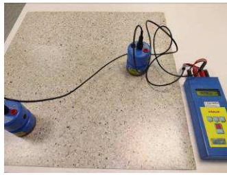
Deposited on a conductive surface ESD PVC PU sealer Transparent type – R pp – 3. Minta
