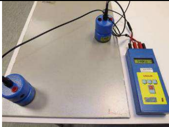
Deposited on a conductive surface ESD Epoxy PU sealer Transparent type – R pp – 8. Minta
