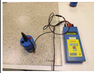
Deposited on a conductive surface ESD PVC PU sealer Transparent type – R g – 3. Minta
