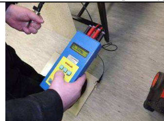
Deposited on a conductive surface ESD Epoxy PU sealer Colored type - R sys – 7. Minta
