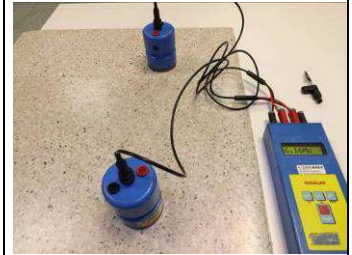
Deposited on a conductive surface ESD PVC PU sealer Between the original surface and the treated surface PU Transparent type – R pp – 3. Minta
